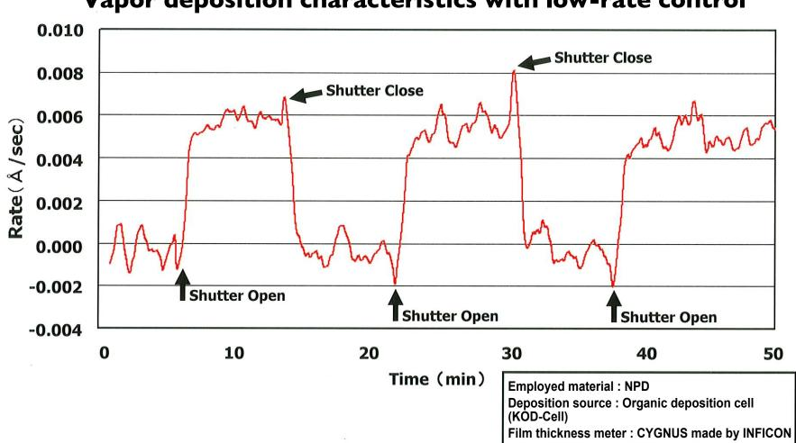
Vapor deposition characteristics with low-rate control
